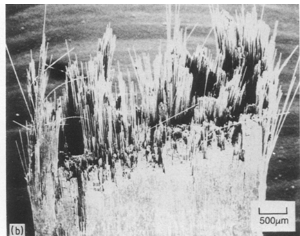
Figure 2 Comparison between tension and flexure behaviour for uniaxial HMU fibre-reinforced 7740 glass: (a) tensile, UTS = 839 MPa (122 ksi); (b) flexure, \sigma = 1150 MPa (166 ksi).
